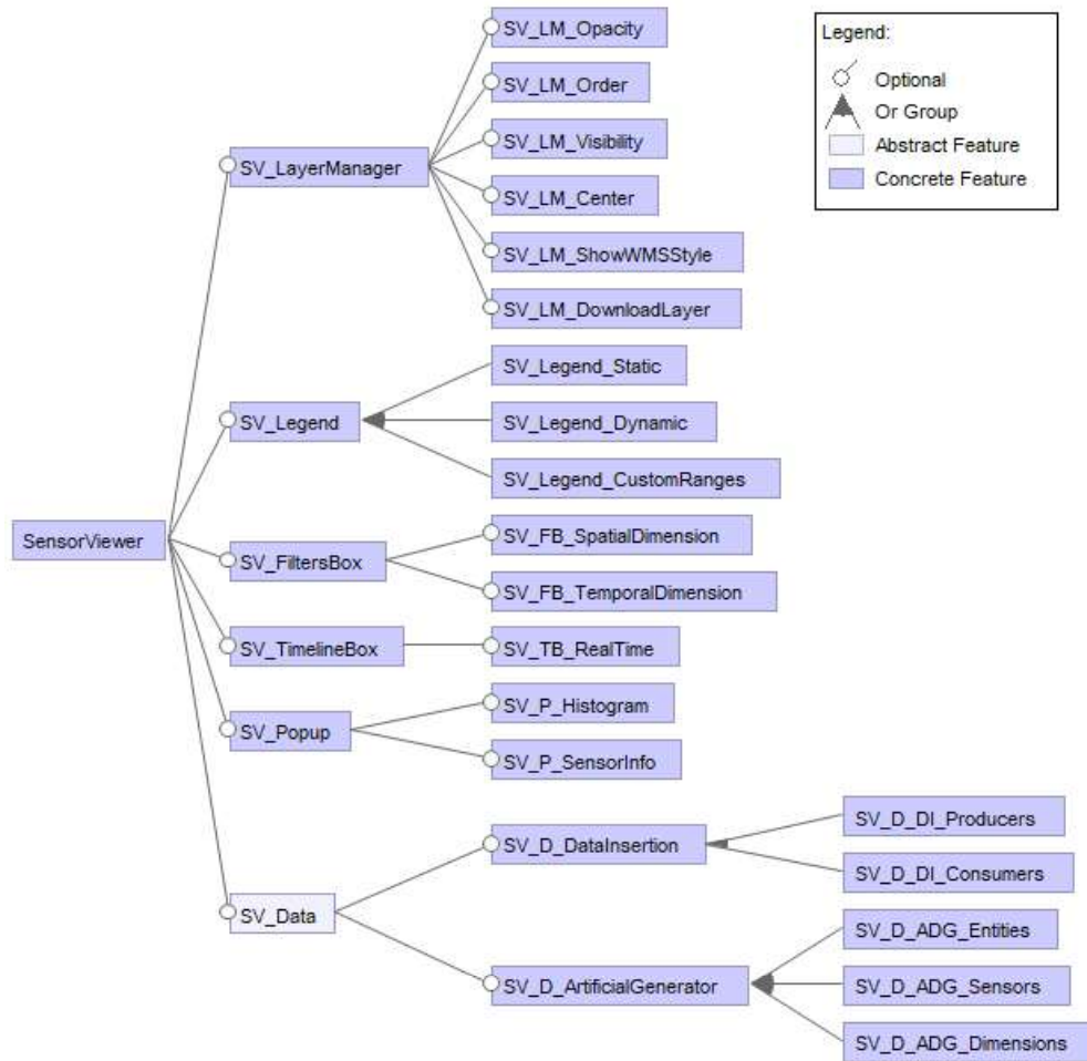
Figure 11: Feature Model of the IoT data warehouse SPL
